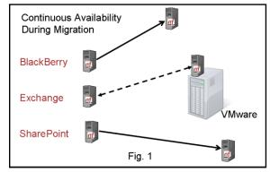
or other work be required on the primary servers. Neverfail does not rely on shared storage architectures; instead, it uses advanced replication technology to maintain cloned system and data copies locally or remotely. Therefore, it can be relied upon for protection against disasters. It also comes into its own as part of a physical-to-virtual (P2V) process as highlighted previously.
